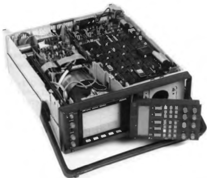
Figure 16.3 Measuring the front unit working condition
